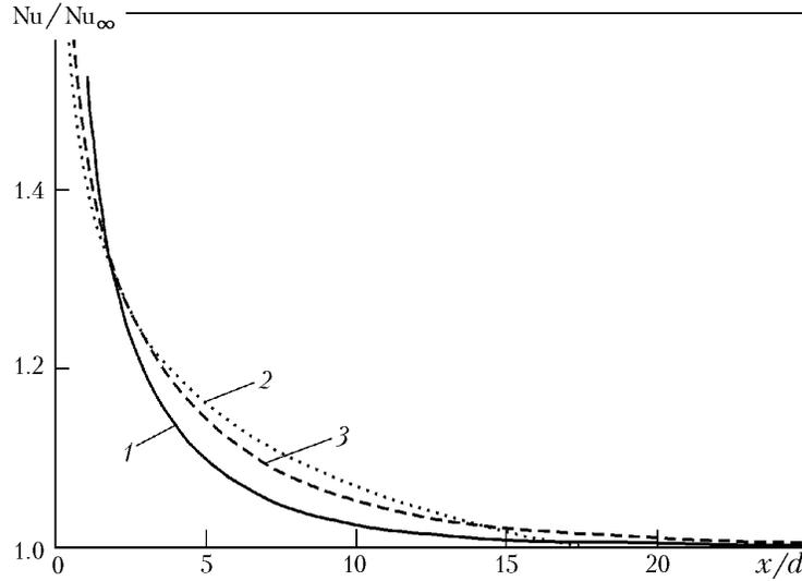
Fig. 3. Change in the local Nusselt number on the initial thermal portion of a circular pipe as a function of  $x/d$ : 1) calculation from (25); 2) (28); 3) (29).
