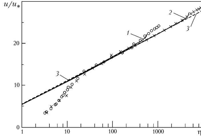
Fig. 1. Dimensionless velocity profiles  $u/u_*$  in the case of turbulent air flow in a circular pipe: 1 and 2) calculation from formulas (8); 3) logarithmic profile (9) for  $\kappa = 0.41$  and  $C = 5.5$  (1)  $Re = 40,260$ ; 2 and 3) 429,200); points, experimental results [4].
